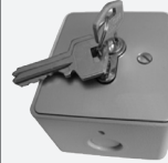
Art. nr. 504903 Standard control element for secure use of one to two drives. Die-cast metal housing with aluminium front plate, IP 54, design 2-sided pressing incl. Standard cylinder lock with 3 keys. double-keyed (NC contacts 300V, 5A), W70xH80xD47mm
