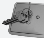
Art. nr. 504904 Standard control element for secure use of one to two drives. Die-cast metal housing with aluminium front plate, IP 54, design 2-sided pressing incl. Standard cylinder lock with 3 keys. double-keyed (NC contacts 300V, 5A), W70xH80xD47mm
