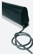
Art. nr. 504900 Safety edges for ohmic evaluation 8.20 kOhm. EPDM; Profile (WxH) 35 x 65 mm on C-profile rail 35 x 14 mm
