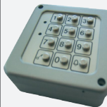
Art. nr. 504905 Shockproof AP housing, IP54, approx. 81x81x30mm, similar to RAL 9007. Buttons and control panel of VA. Tamper-proof design. Power supply over 9V block (included). 3 channels for individual 2-6 digit code; 1 channel for free use (e.g., for lighting).
